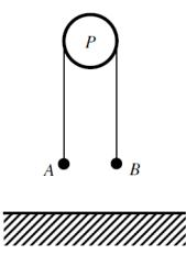
Two particles A and B of respective masses 3 kg and m kg are each attached to the two ends of a light inextensible string which passes over a smooth pulley P. The two particles are held at rest, both at a height of 1.28 m above a horizontal floor with the portions of the strings not in contact with the pulley vertical.
