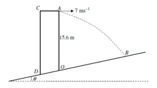
The figure above shows the cross section of a vertical tower *OACD* standing on a plane inclined at an angle  $\theta$  to the horizontal, where  $\tan \theta = 0.1$ .
