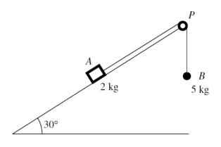
Two particles A and B, of mass 2 kg and 5 kg respectively, are attached to each of the ends of a light inextensible string. The string passes over a smooth pulley P, at the top of a fixed rough plane, inclined at  $30^{\circ}$  to the horizontal.
