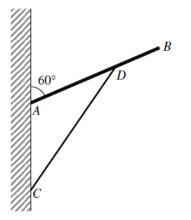
The figure above shows a uniform rod AB, of weight  $\sqrt{3}W$  and length 4L, is freely hinged at the end A to a vertical wall.
