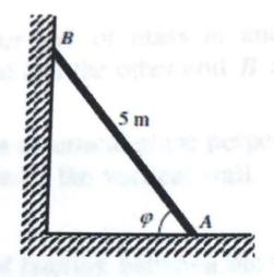
The figure above shows a ladder AB resting in equilibrium with one end A on rough horizontal ground and the other end B against a smooth vertical wall. The ladder is modelled as a uniform rod of length 5 metres and mass  $20 \, \text{kg}$ , and lies in a vertical plane perpendicular to the wall and the ground, inclined at an angle  $\varphi$  to the horizontal.
