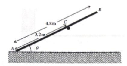
The figure above shows a plank AB resting on a smooth peg. The plank is modelled a uniform rod of weight W N and of length 4.8 metres, resting on the peg at the point C, where AC is 3.2 metres.
