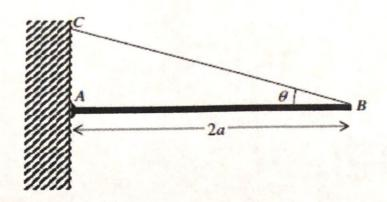
The figure above shows a uniform rod AB of length 2a and of mass m smoothly hinged at the point A, which lies on a vertical wall.
