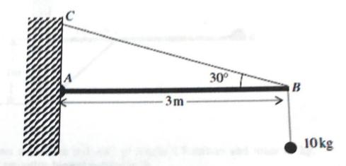
The figure above shows a uniform rod AB of length 3 metres and of mass 20 kg smoothly hinged at the point A, which lies on a vertical wall. A particle of mass 10 kg is suspended from the end B of the rod. The rod is kept in a horizontal position by a light inextensible string BC, where C lies on the same wall vertically above A.
