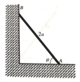
The figure above shows a uniform ladder AB of length 2a and of mass m resting with the end A on rough horizontal ground and the end B against a smooth vertical wall. The ladder is inclined at an angle  $\theta$  to the ground.
