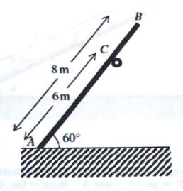
The figure above shows a uniform rod AB of length 8 metres and of mass 15kg. The rod is resting in equilibrium with the end A on rough horizontal ground and the point C, where AC = 6 metres, on a smooth peg. The rod is inclined at  $60^{\circ}$  to the ground.
