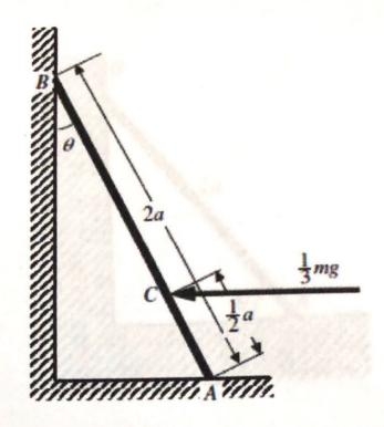
A ladder of length 2a and mass m, has one end A on smooth horizontal ground and the other end B against a smooth vertical wall.
