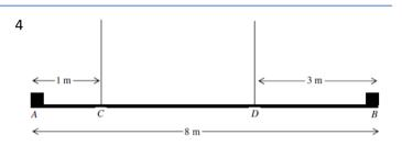
A uniform iron girder AB has length 8 m and weight W N. A load of 250 N is attached to the girder at A and a load of 400 N is attached to the girder at B.
