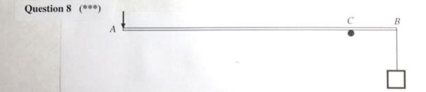
A mechanical lever consists of a uniform steel rigid rod AB, of length 2 m and weight 100 N, placed over a smooth pivot at C.
